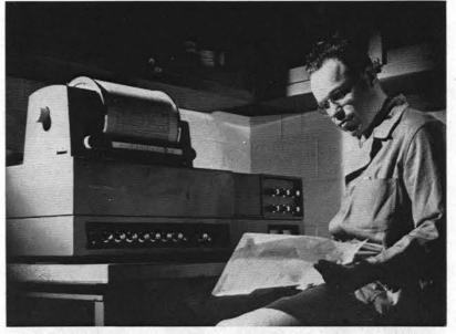
BOB KELLEY (8115-2) studies a "fingerprint" made by the infrared spectrophotometer. Spectrophotometers are used to identify foreign elements or impurities which might cause malfunction.
